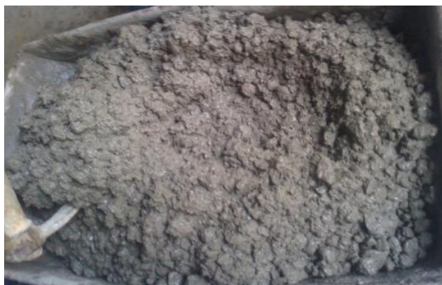
Figure 1. Fresh GPC Concrete
