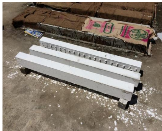
Figure 6. Beams after 28 days of curing with white wash
