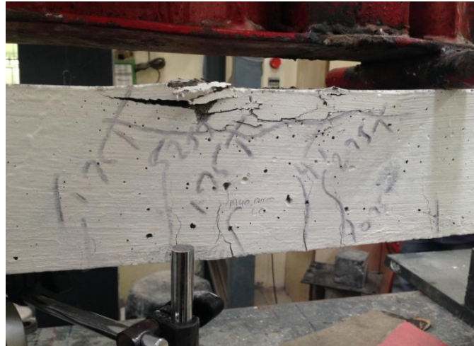
Figure 7. Crack pattern of beam
