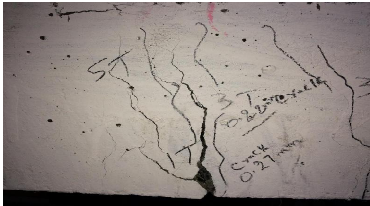
Figure 8. Crack width and Crack pattern of the 50 mm clear cover of M25 grade of concrete beam
