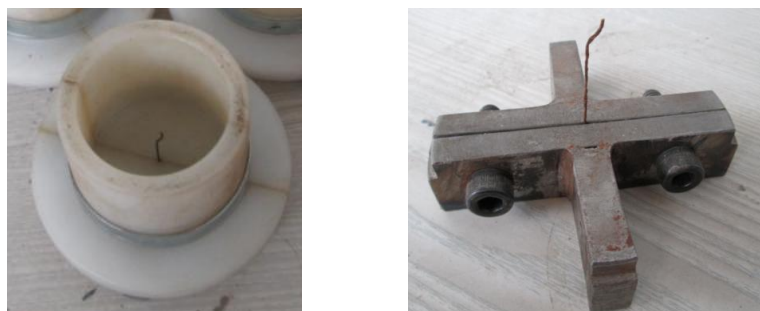
Figure 5. Fiber pull-out specimen mold
