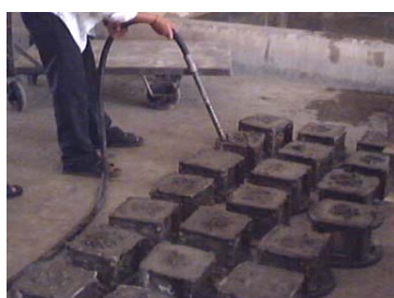
Figure 2. Details of re-vibration of concrete
