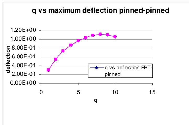
Figure 4. Comparison of  $q$  vs. maximum transverse deflection for EBT and TBT for pinned-pinned boundary conditions
