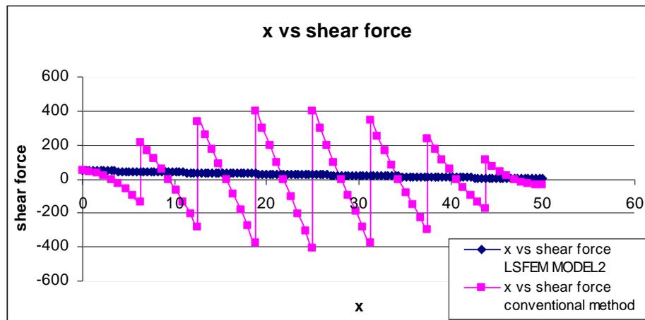
Figure 5. Comparison of x vs. shear force for LSFEM MODEL2 and conventional model
