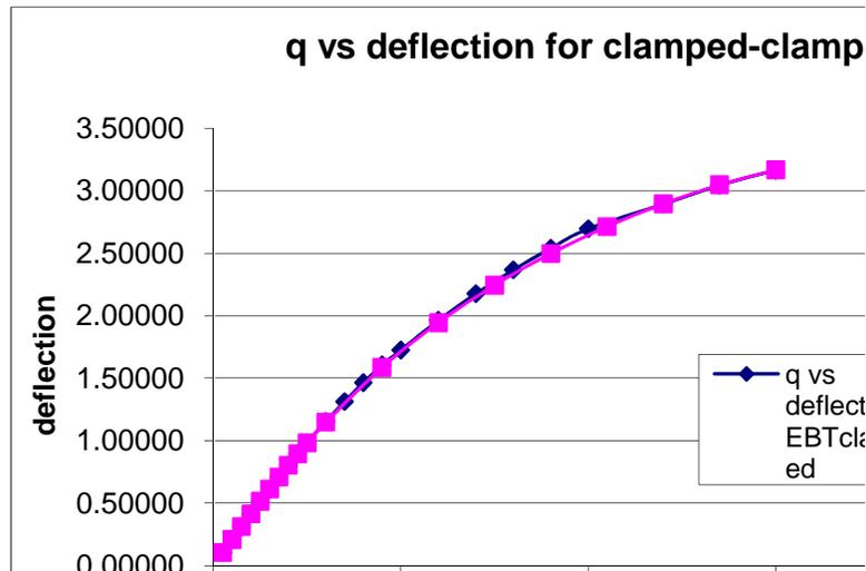
Figure 3. Comparison of  $q$  vs. maximum transverse deflection for EBT and TBT for clamped-clamped boundary conditions
