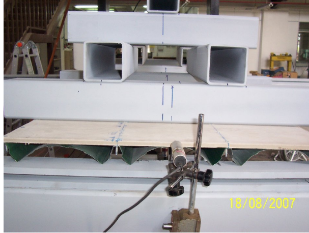
Figure 6. Buckling of lower flange of Ajiya CL660
