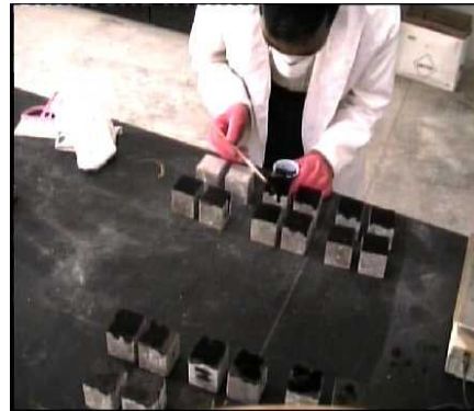
Figure 6. Painting concrete surface
