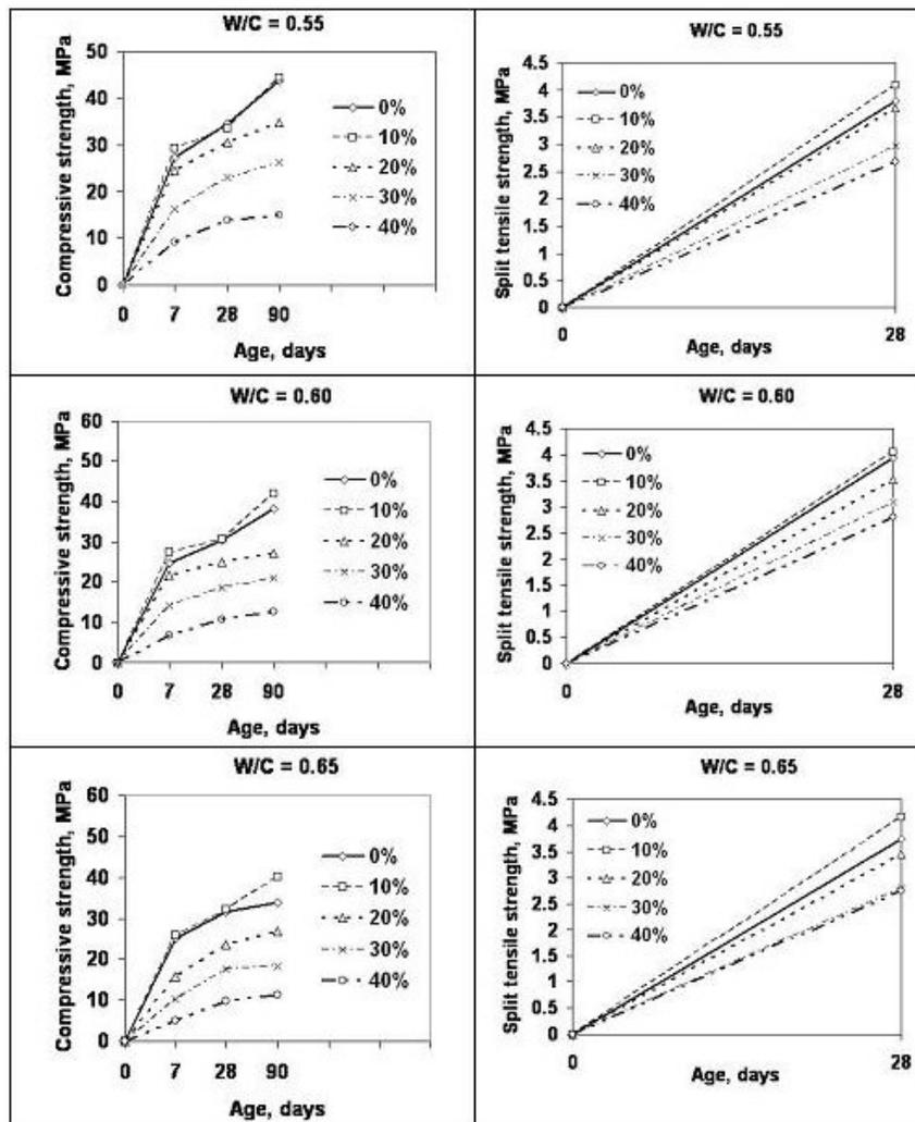
Figure 2. Variation of compressive and split-tensile strengths versus age using different percentage replacements of phosphogypsum with water-binder ratios 0.55, 0.60 and 0.65
