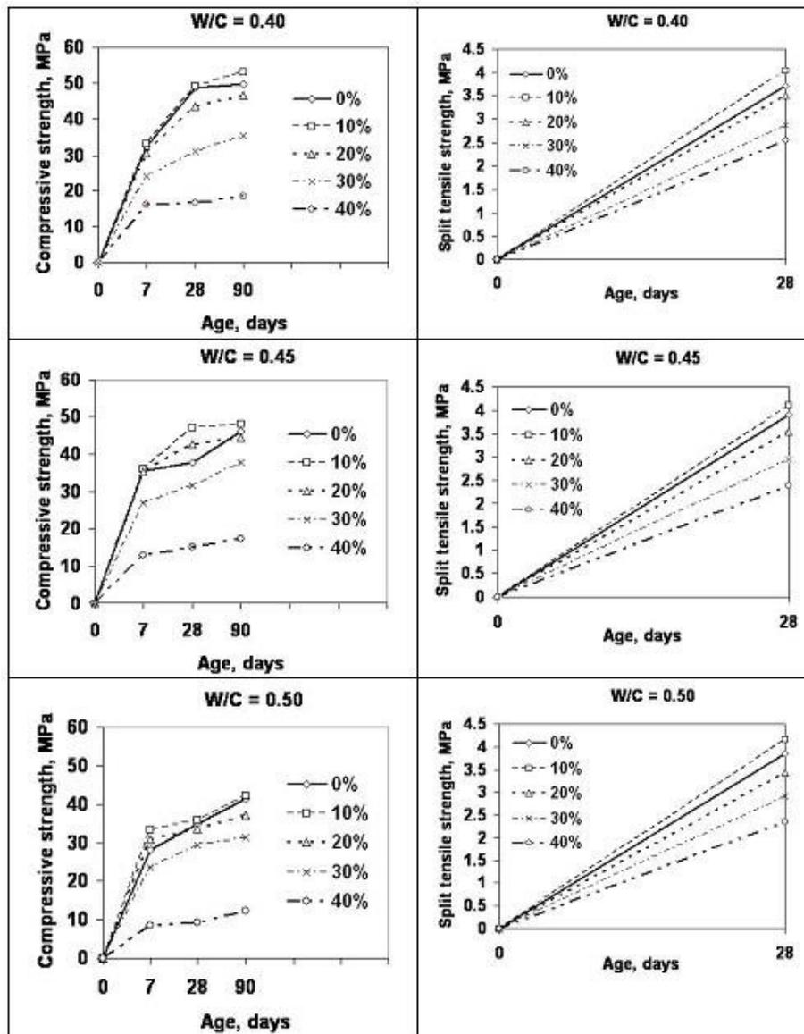
Figure 1. Variation of compressive and split-tensile strengths versus age using different percentage replacements of phosphogypsum with water-binder ratios 0.40, 0.45 and 0.50
