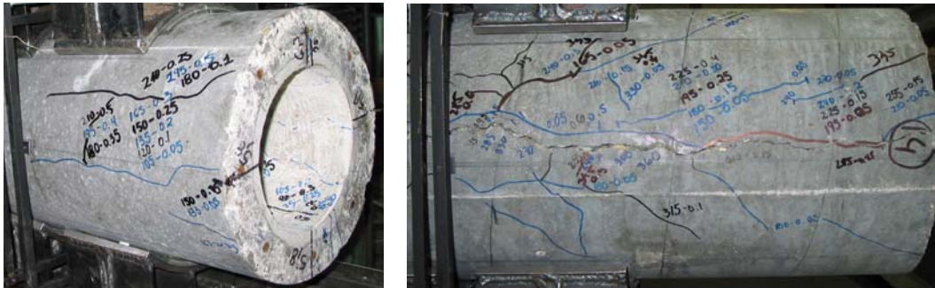
Figure 2. Crack pattern of a short (EB1) and of a long specimen (EB8)
