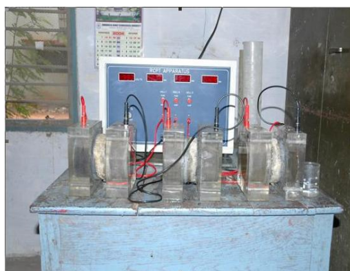
Figure 2. Chloride ion permeability test setup
