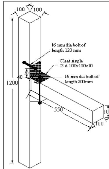
Figure 3. Precast beam-column connection using cleat angle
