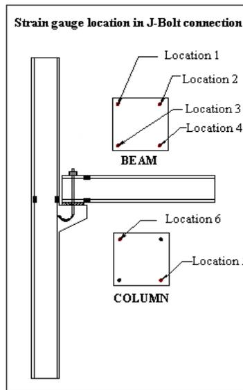
Figure 7. Strain gauge locations in J-bolt connection
