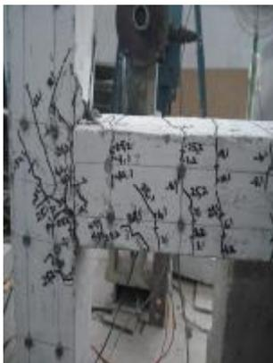
Figure 9. Failed monolithic specimen
