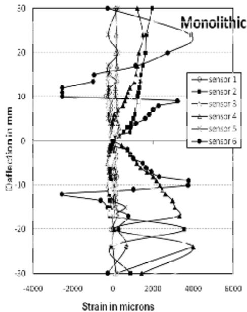
Figure 16. Strain in reinforcements in specimen ML
