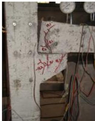
Figure 10. Failed J-bolt connection
