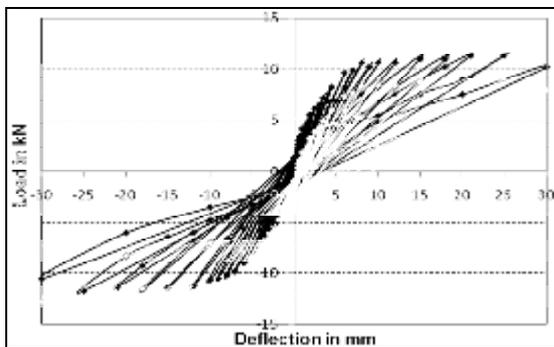
Figure 12. Hysteresis curve for monolithic specimen ML
