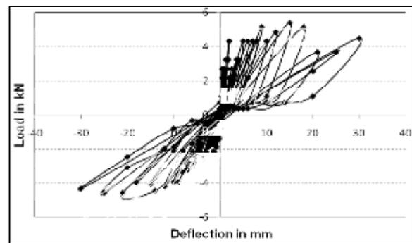
Figure 13. Hysteresis curve for precast specimen PC1
