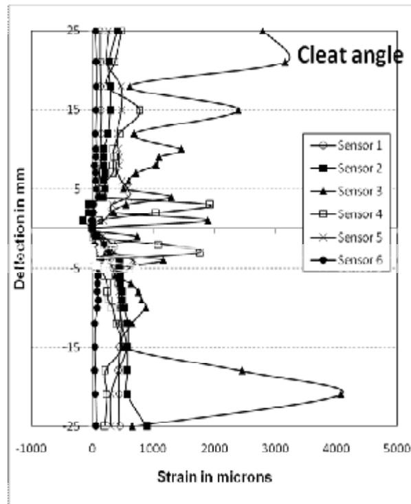
Figure 18. Strain in reinforcements in specimen PC2
