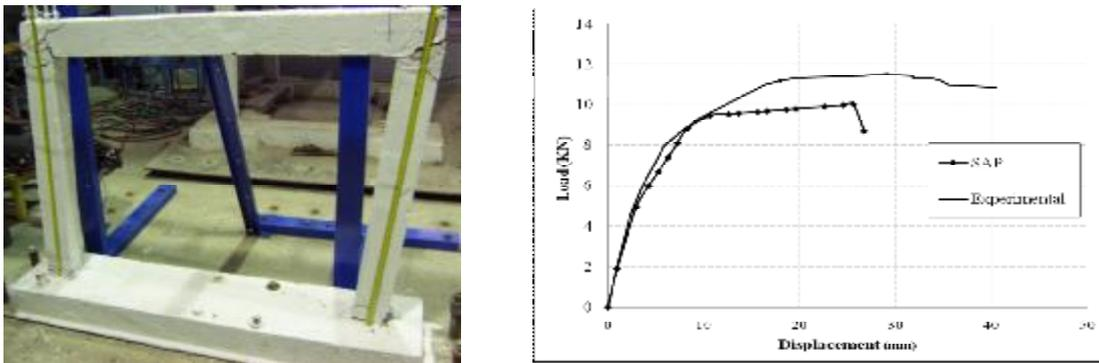
Figure 3. The BF model after pushover testing and its pushover curves
