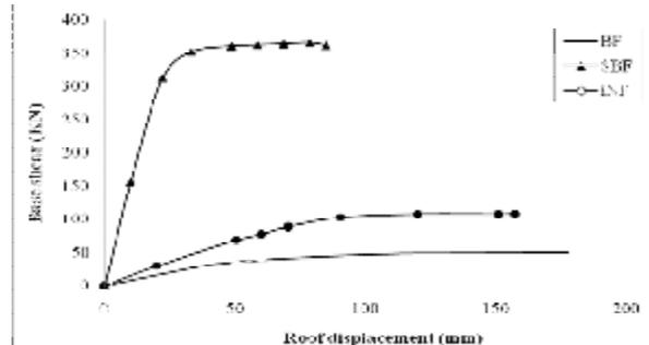
Comparison of pushover curves before and after the retrofitting of the frame designed as per Sequence 3
