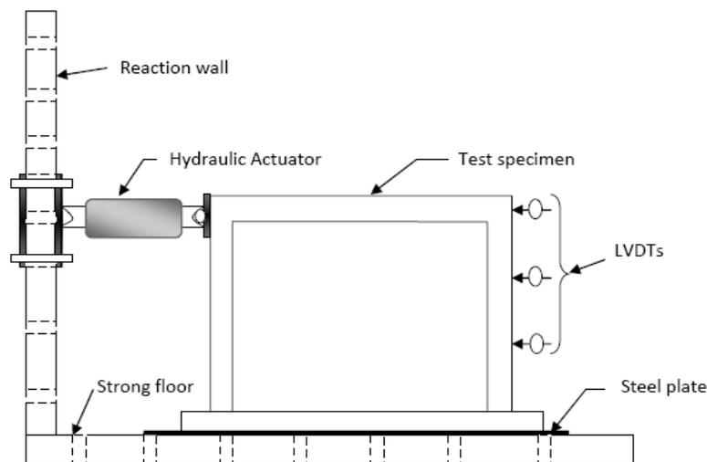
Figure 2. The pushover test setup of BF model
