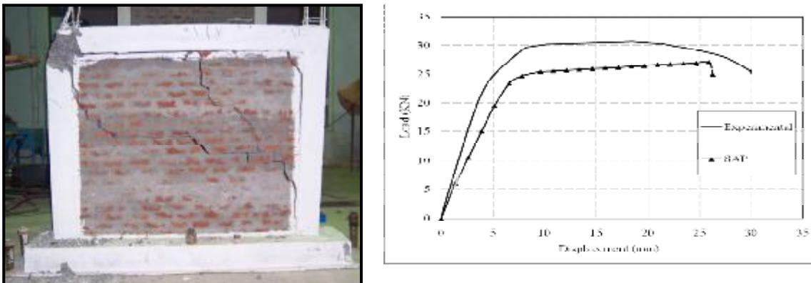
Figure 4. The IBF model after pushover testing and its pushover curves
