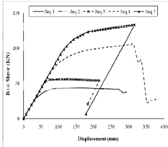
Figure 9. Pushover curves of 4-storey RC frame building designed with different IS codes
