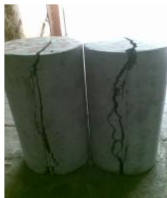
Plate 4. Cracking pattern of cylinders
