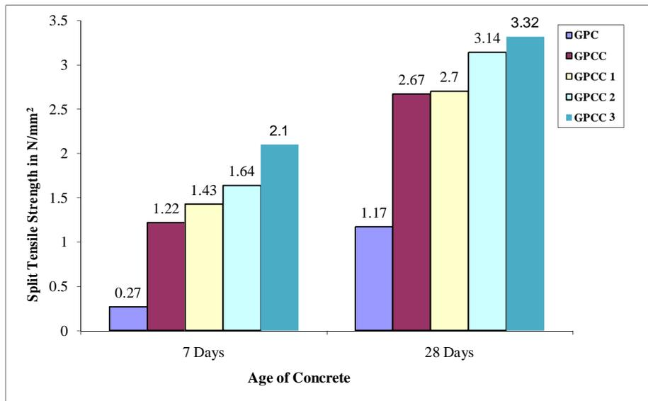
Figure 3. Effect of addition of steel fibres on split tensile strength
