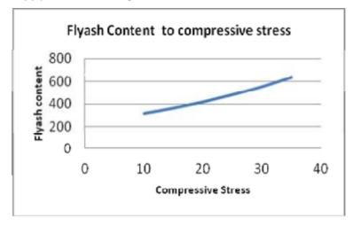
Figure 1. Shows flyash content to the compressive strength
