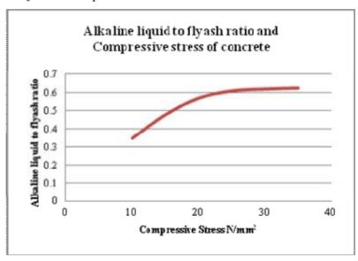
Figure 2. Generalised relation between free alkaline liquid to flyash ratio and compressive strength of concrete
