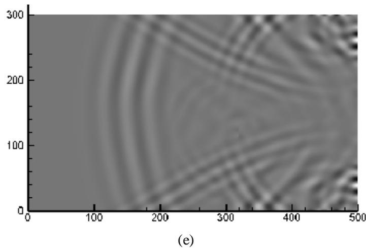
Figure 11. Horizontal displacement contours of cracked steel plate drawn in five various time steps of (a) 30  $\mu\text{sec}$ , (b) 45  $\mu\text{sec}$ , (c) 60  $\mu\text{sec}$ , (d) 67.5  $\mu\text{sec}$ , and (e) 82.5  $\mu\text{sec}$
