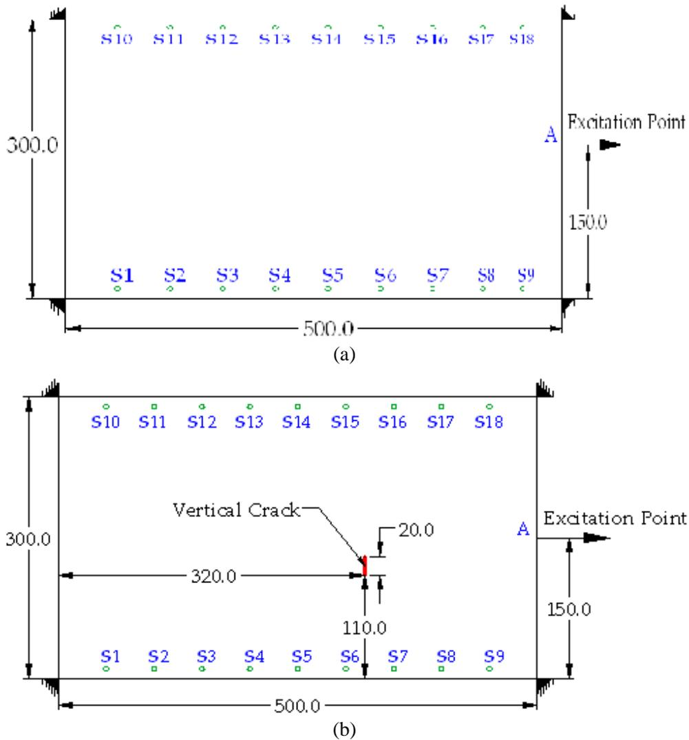
Figure 9. Geometry, loading, boundary conditions, and sensor alignment of the plate of the second example (length unit is in millimeters): (a) uncracked plate, (b) cracked plate
