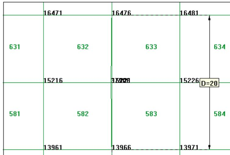
Figure 10. A structured mesh on the cracked steel plate of the second example depicted using GID: (a) rectangular domain with an embedded crack, (b) detailed view of cracked zone
