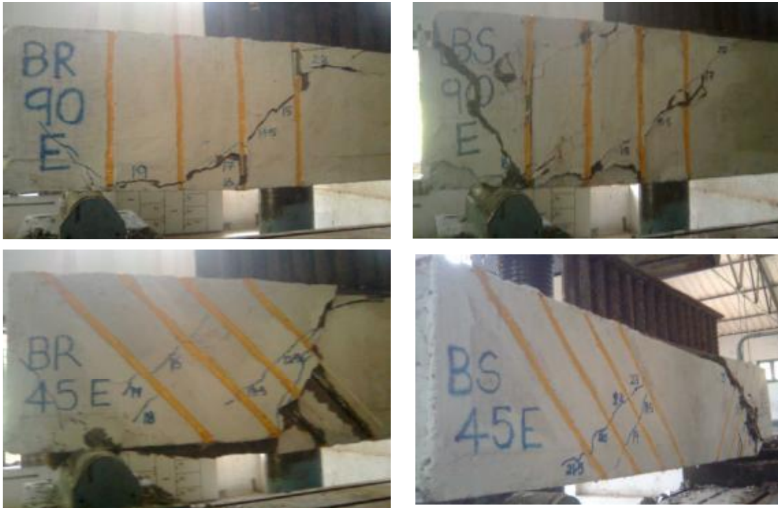
Figure 1. Crack pattern of specimen in series S1
