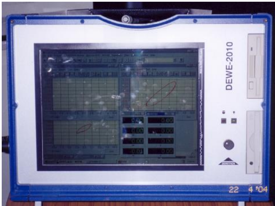
Figure 11. View of the energy dissipation hysteretic curves as observed from the steady state dynamic test on the RC frame structure under study
