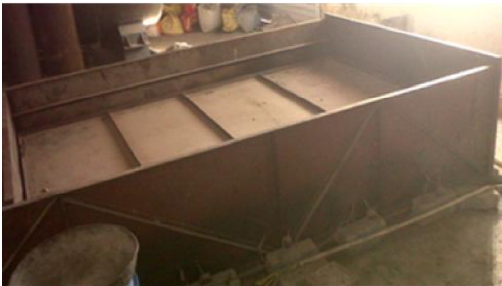
Figure 3. Heat curing chamber under operation mode
