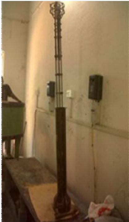
Figure 4. Specimen (typical) during table vibration
