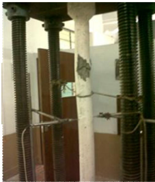
Figure 8. Failure pattern of G50 concrete column (typical)
