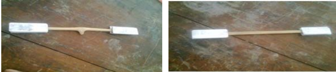
Figure 1. Tension test specimen with and without node, with end tabs
