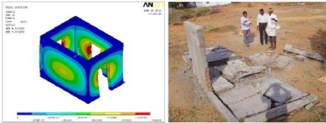
Figure 2. Performance of brick walls – ANSYS model and actual behaviour
