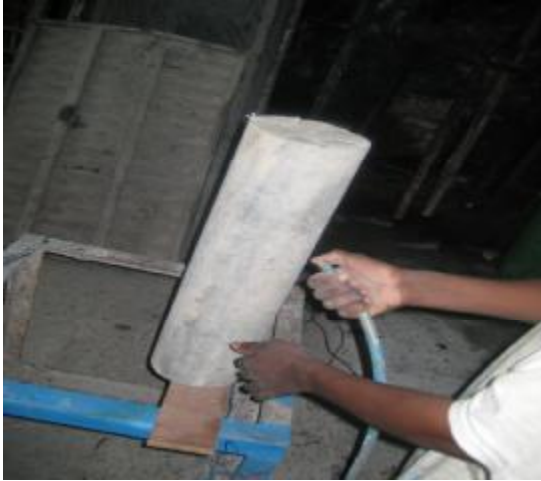
Figure 1. Air-cleaning under progress
