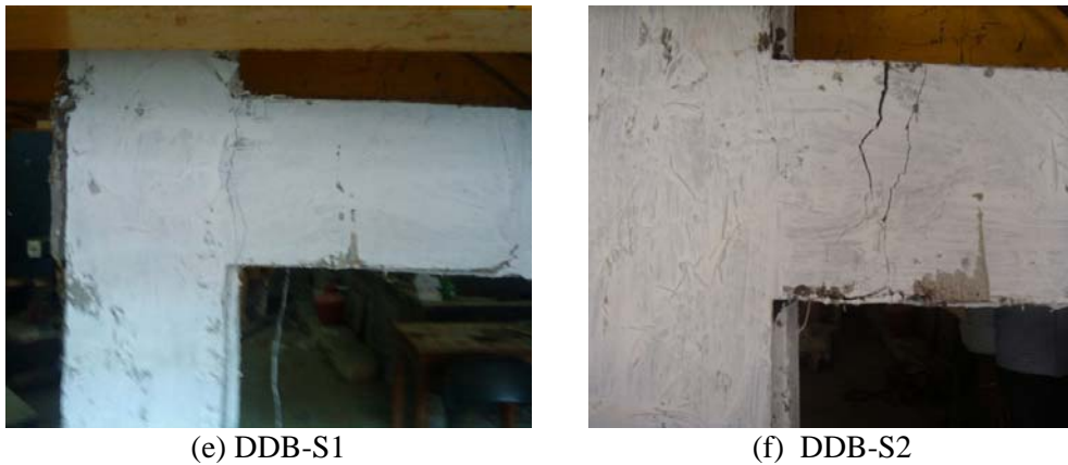
Figure 10. Crack pattern of tested beam column joints
