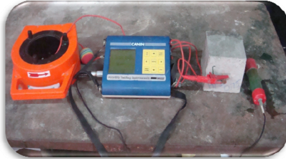
Figure 14. Half-cell potential test setup
