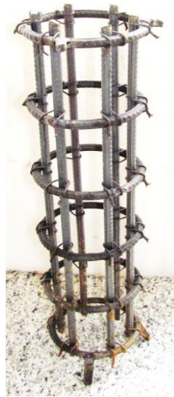
Figure 1. Internal steel reinforcement
