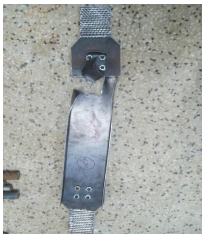
Figure 7. Block shear failure
