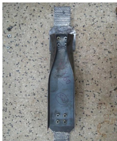
Figure 8. Net section failure
