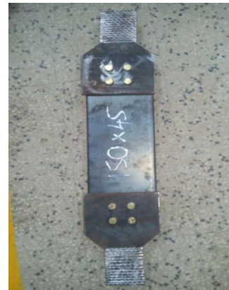
Figure 3. Channel section of 150x45x2mm
