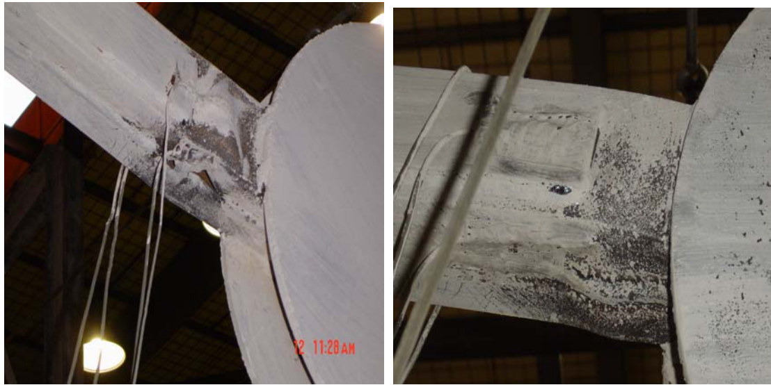
b) Buckling of flange lip in Model 1100-3 c) Local buckling of flange in Model 1100-4
