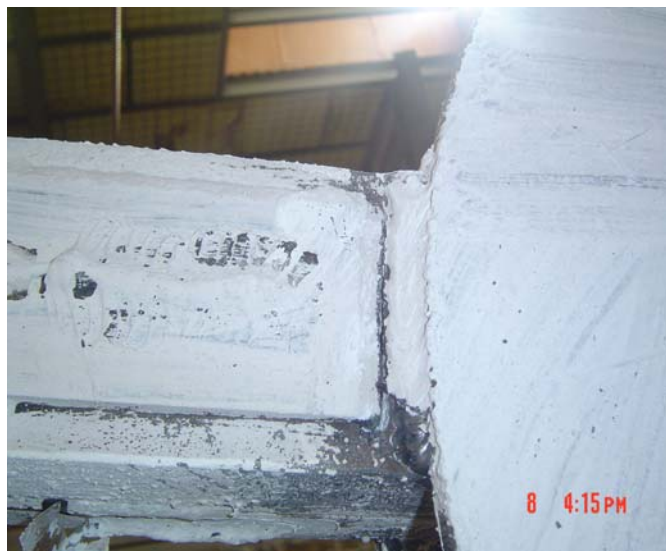
a) Fillet weld fracture in Model 1100-2
