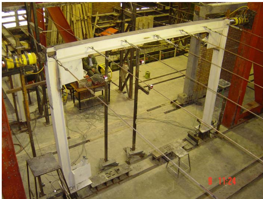
Image 4. Bare Frame under lateral cyclic loading
