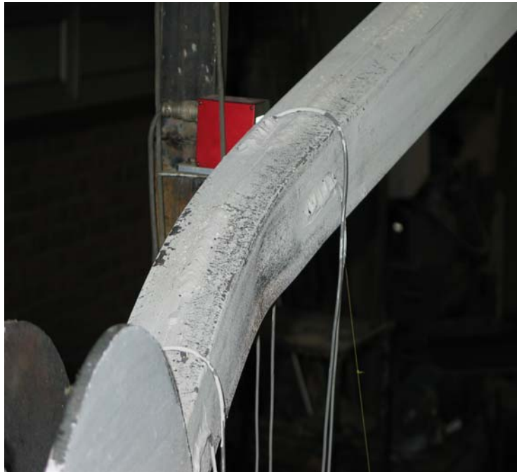
Image 2. Plastic hinge due to buckling in model 1600
