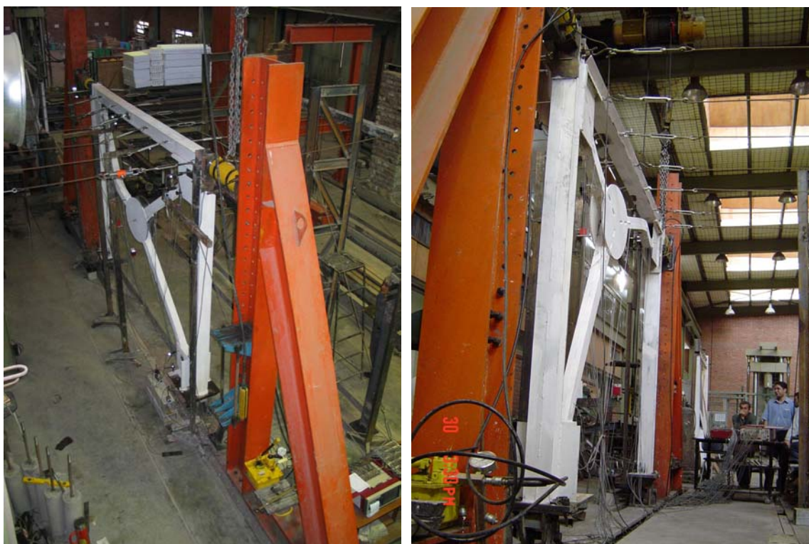
Image 1. Set up of tests and buckling of longest member of bracing
