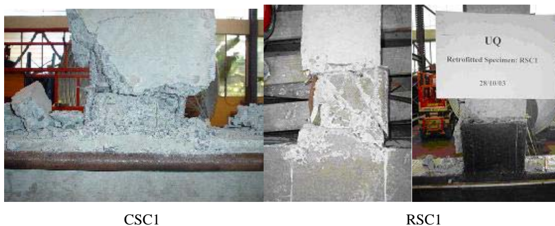
Figure 11. Failure pattern of specimens CSC1 and RSC1.
