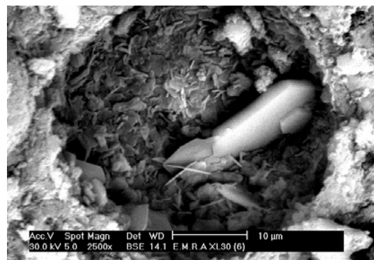
e) SEM micrograph of OPC cement paste at 400°C
