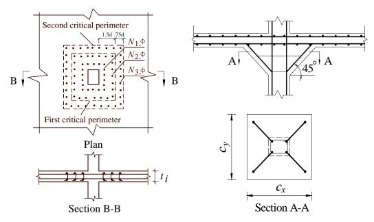
Figure 3. Shear reinforcement around columns
