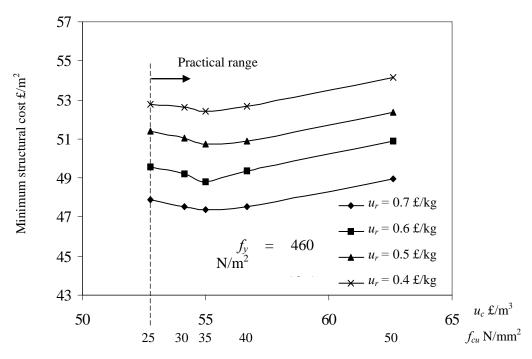
(c)  $u_c$  changes with respect to  $f_{cu}$  according to Hansons company prices (Case 3) Figure 8. The minimum structural cost versus the unit cost of concrete
