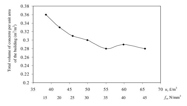
Figure 9. Variation of the total volume of concrete in the optimum structure per unit area of the building versus the unit cost of concrete and concrete strength
