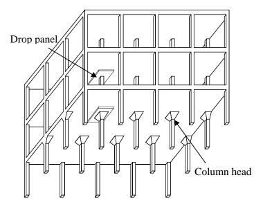
Figure 1. A typical flat slab building
