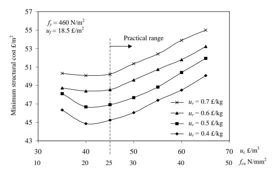
a) u<sub>c</sub> changes with respect to f<sub>cu</sub> linearly (Case 1)
