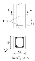
Figure 5. Details of a typical column
