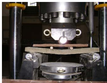
Figure 6. Flexural strength test setup
