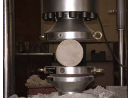
Figure 5. Split tensile strength test of a cylinder
