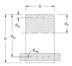
Figure 2. Equivalent transformed cross section
