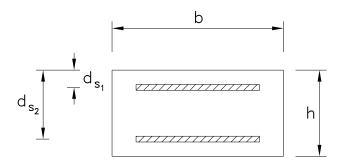
Figure 8. Cross-section of one-way reinforced concrete slab
