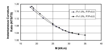
Figure 12. Comparison the effect of reinforcement percentage (P=1%)
