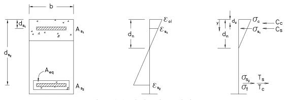
Figure 4. Cracked section analysis
