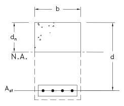
Figure 1. Average section after cracking
