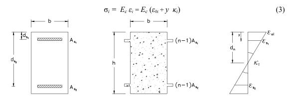
Figure 3. Uncracked section analysis
