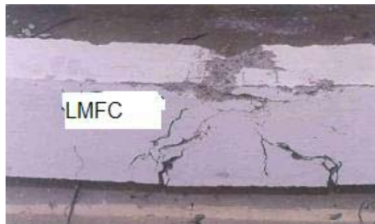
Figure 4. Typical hinged beams-failure pattern under monotonic loading
