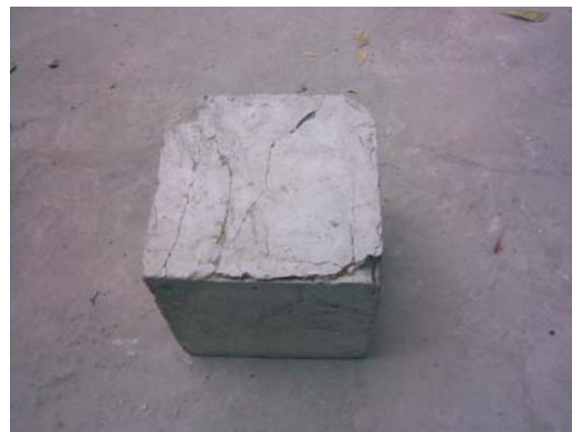
Figure 8. Failure pattern of fiber reinforced concrete cube
