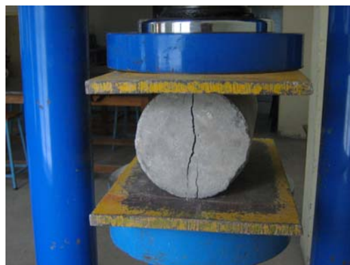
Figure 10. Failure pattern of plain concrete cylinder
