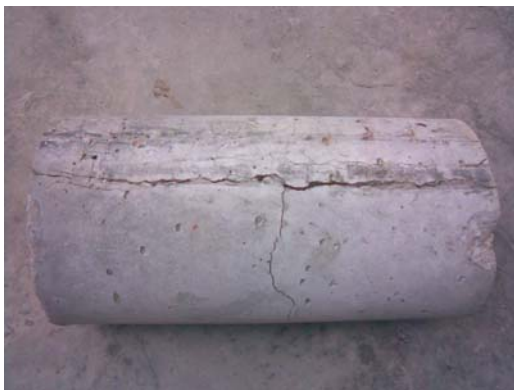
Figure 7. Failure pattern of fiber reinforced concrete cylinder
