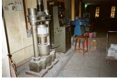
Plate 4. Compressive strength test
