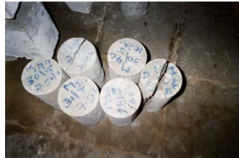
Plate 6. Tested specimens (splitting tensile strength)
