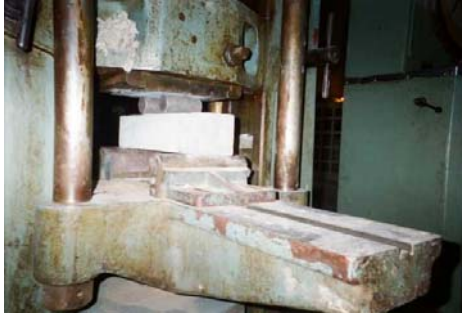
Plate 3. Flexural strength test
