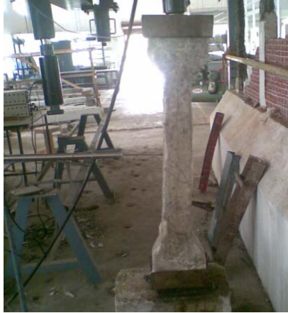
Figure 7. Experimental set up for wrapped short column
