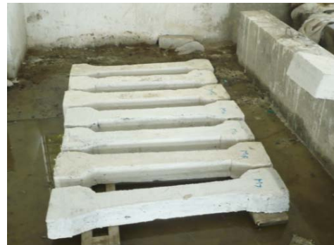
Figure 4. Short column specimens before testing
