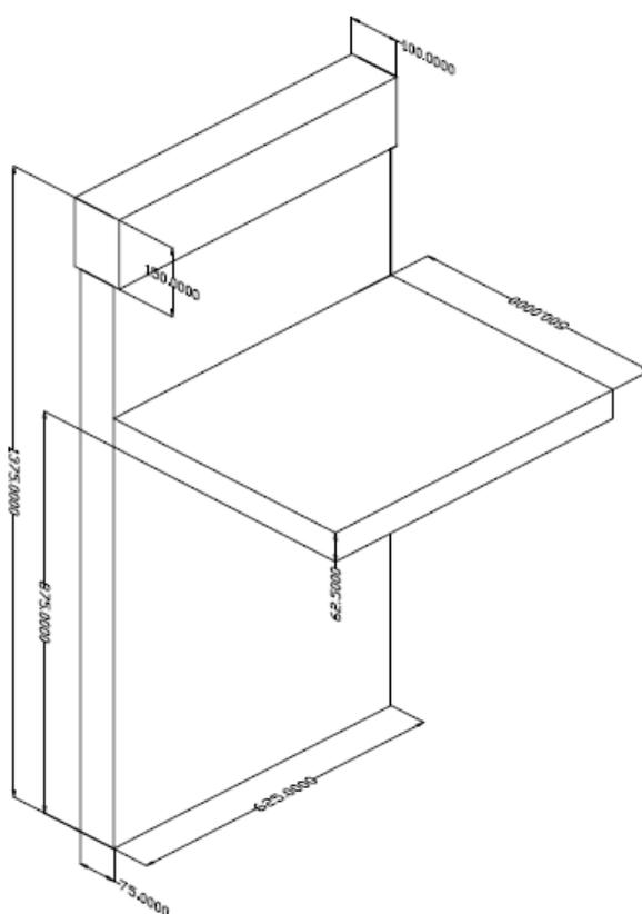
Figure 1. Wall-slab joint (1/4<sup>th</sup> scale model)
