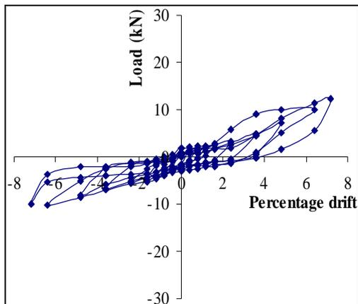
Figure 8. Load – drift hysteretic loop for Type 1 specimen
