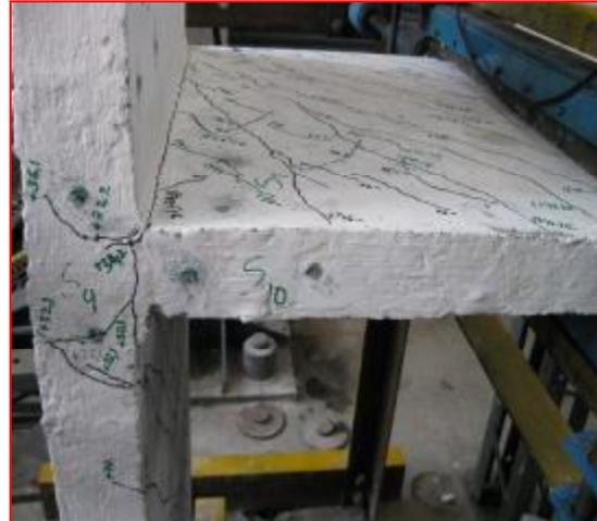
Figure 7. Cracks in Type 2 specimen
