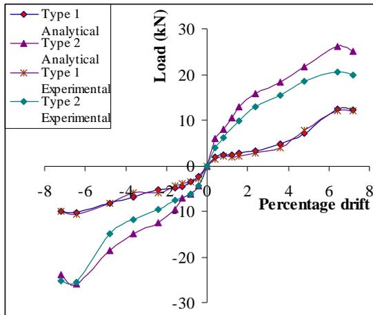
Figure 12. Comparison of load-drift relations of specimens
