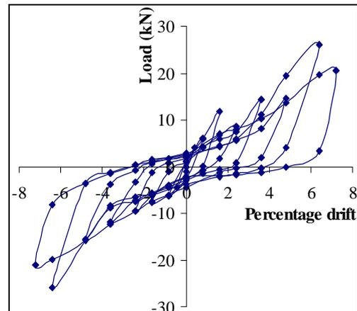
Figure 9. Load – drift hysteretic loop for Type 2 specimen
