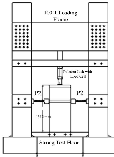
Figure 2. Schematic diagram of test set up
