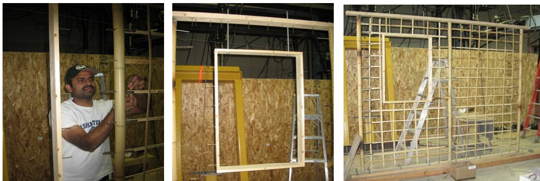
Figure 6. Construction sequence for the 2.44m long test specimen details
