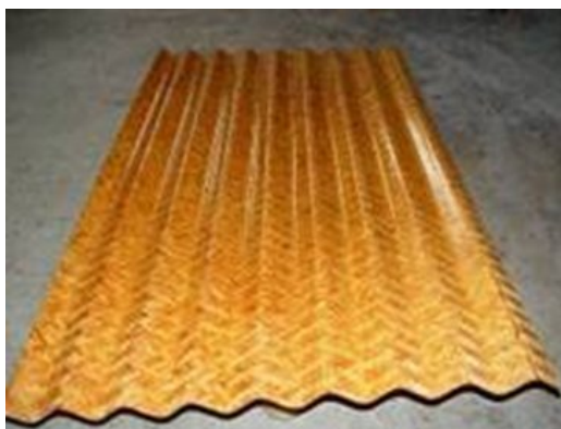
Figure 1. 300 mm×950 mm bamboo mat corrugated sheet
