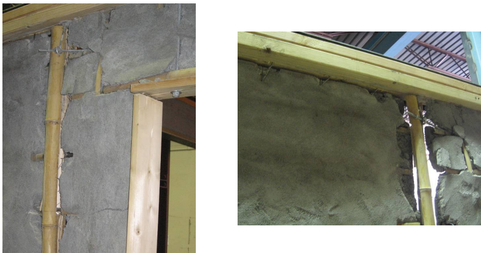
Figure 9. Photographs of failure mechanism for 2.44m long test specimen
