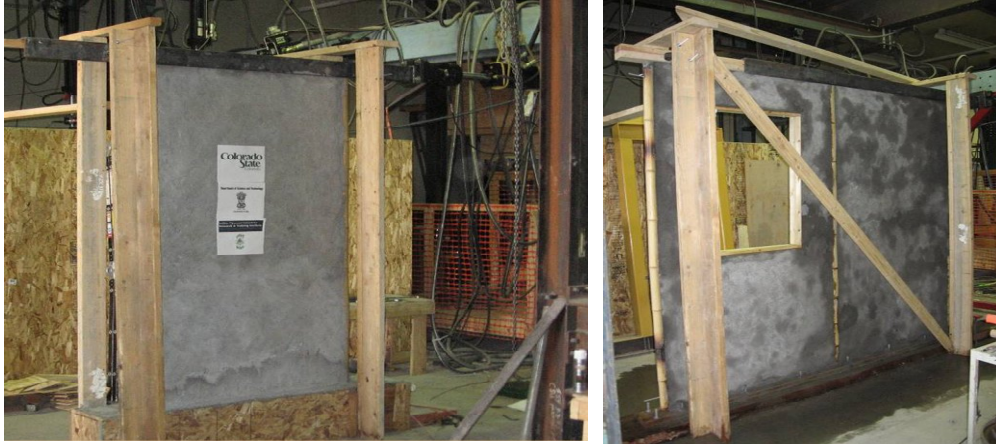
Figure 7. Completed test specimens curing in place
