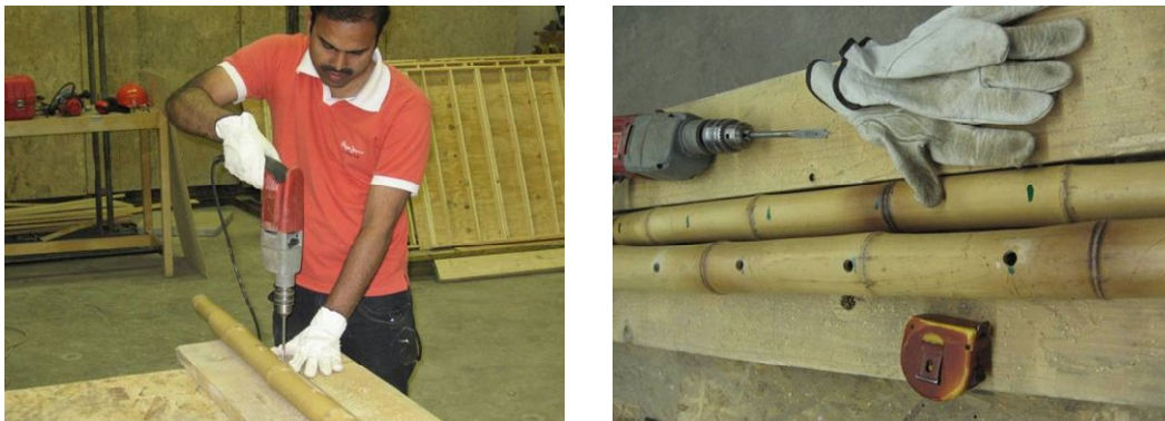
Figure 5. Preparation of bamboo top plate for the 2.44m long test specimen
