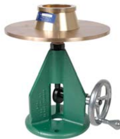
Figure 3. Flow table test setup
