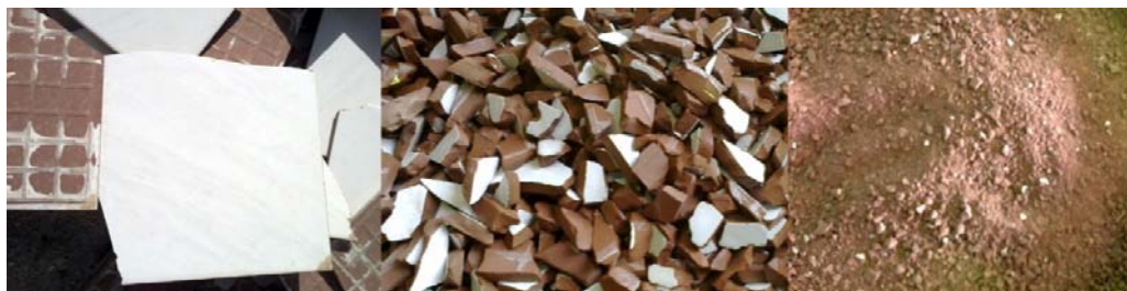
Figure 1. Ground ceramic tile preparation process
