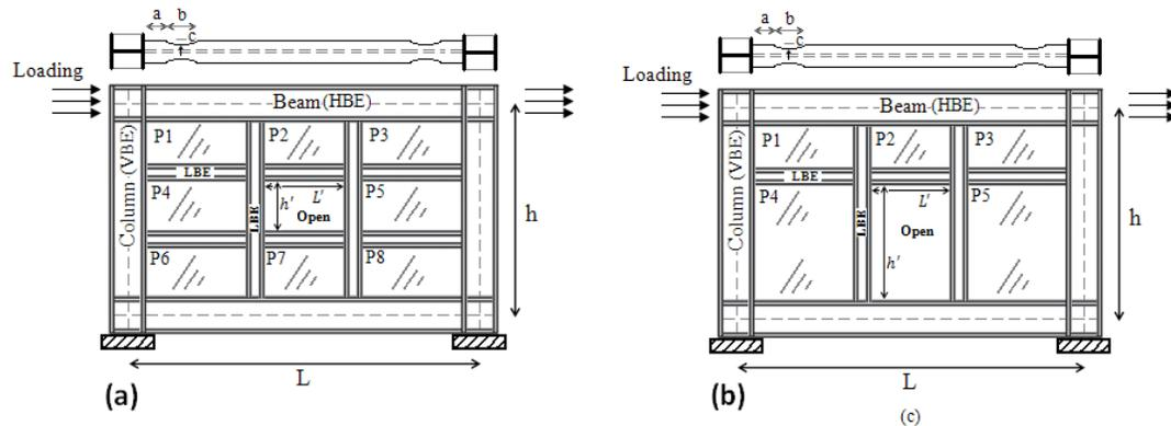
Figure 1. Partial-height rectangular openings studied by Hosseingzadeh and Tehranizadeh, (a) window-type, and (b) door-type openings, adapted from Ref. [10]
