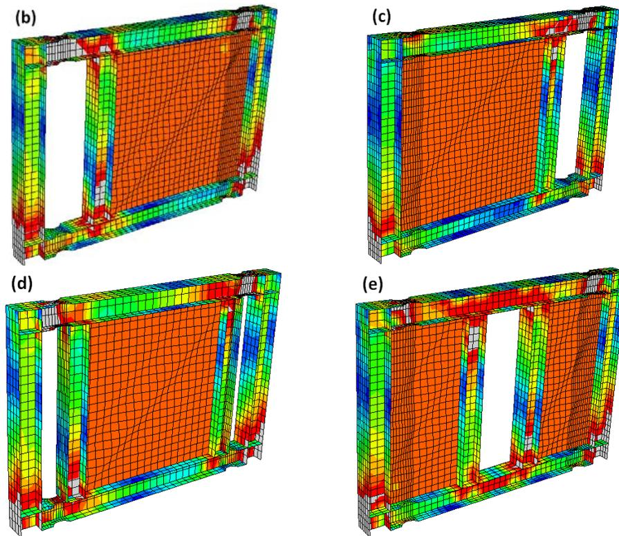
Figure 5. Mises stress distribution of typical SPSWs ( $L/h=1.43$  and  $L'=1$  m), (a) without the openings, and with the openings of, (b) L, (c) R, (d) LR, and (e) M configurations, at the ultimate state
