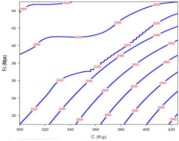
Figure 2. Contour of water with the compressive strength and the cement obtained from Eq. (11)
