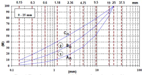
Figure 1. Fine and coarse aggregate gradation curve for maximum size = 25mm
