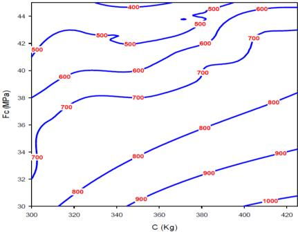
Figure 3. Contour of fine aggregate with F<sub>c</sub> (MPa) vs. Cement (Kg) value from Eq. (11)
