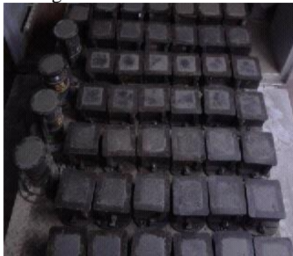
Figure 3. Casting of specimens
