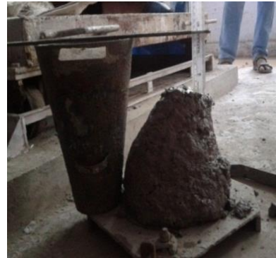
Figure 2. Measuring of slump
